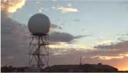
Dual-Polarized Radar greatly improves weather forecasters' ability to predict the type and intensity of precipitation, and where and when it will fall. This new technology is the result of 30 years of research and development by NOAA's National Severe Storms Laboratory. Credit: NOAA..
