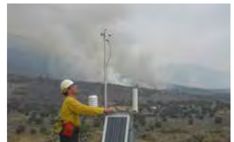
Setting up an Incident Remote Automated Weather Station (IRAWS) during a fire near Hiawatha, Utah. Credit: Alan Hester
