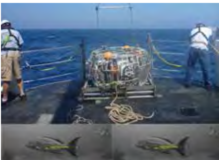
The NOAA Southeast Fisheries Science Center utilizes an array of four stereo video cameras to estimate the abundance of reef fish. Advances in optical technologies have improved the assessments for commercial and recreational stocks in many regions, particularly for stocks that occur in habitats which are inaccessible or vulnerable to conventional sampling gear such as trawls..
