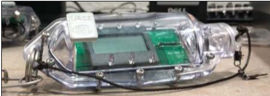
Figure 3. Lindgren Pitman LP Hook Timer HT-600. The plunger on the right side of the hook timer is held in place by a magnet, which once pulled activates a stop watch in the body of the hook timer.
